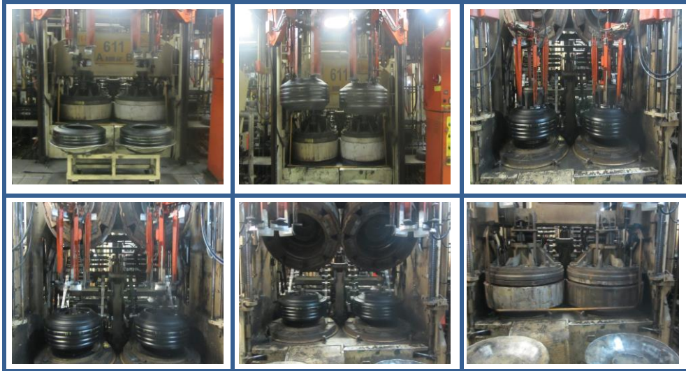
Figure 6. Steps of tire curing process
